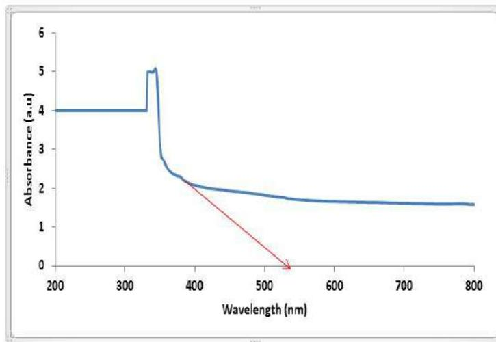
Figure 3. UV Visible absorbance spectra of CdS thin film of deposition time period 24 hours at room temperature
