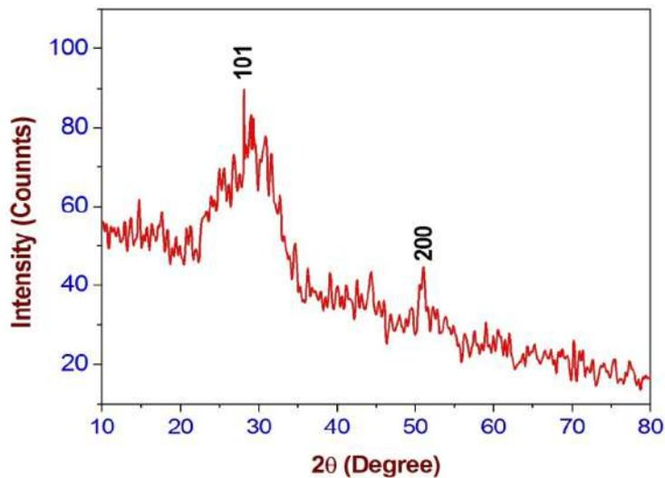
Figure 1. XRD pattern of CdS thin films of deposition time period 12 hours at room temperature
