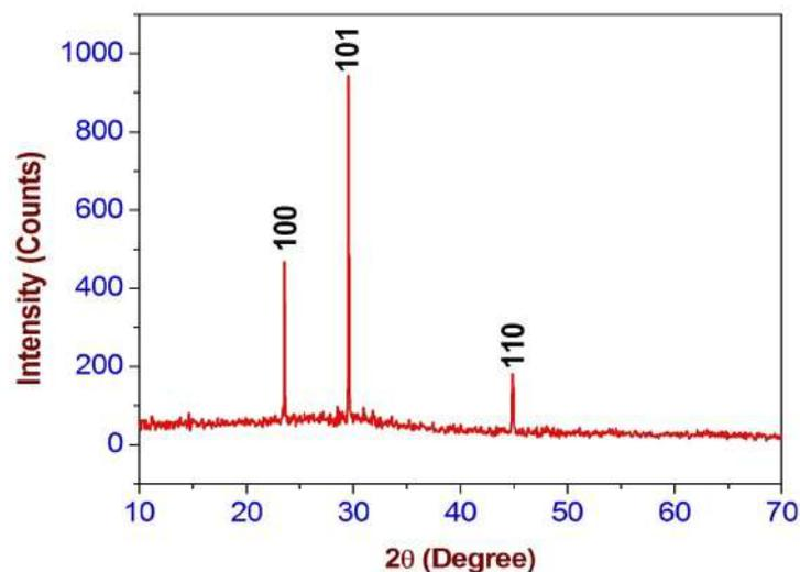
Figure 2. XRD pattern of CdS thin films of deposition time period 24 hours at room temperature
